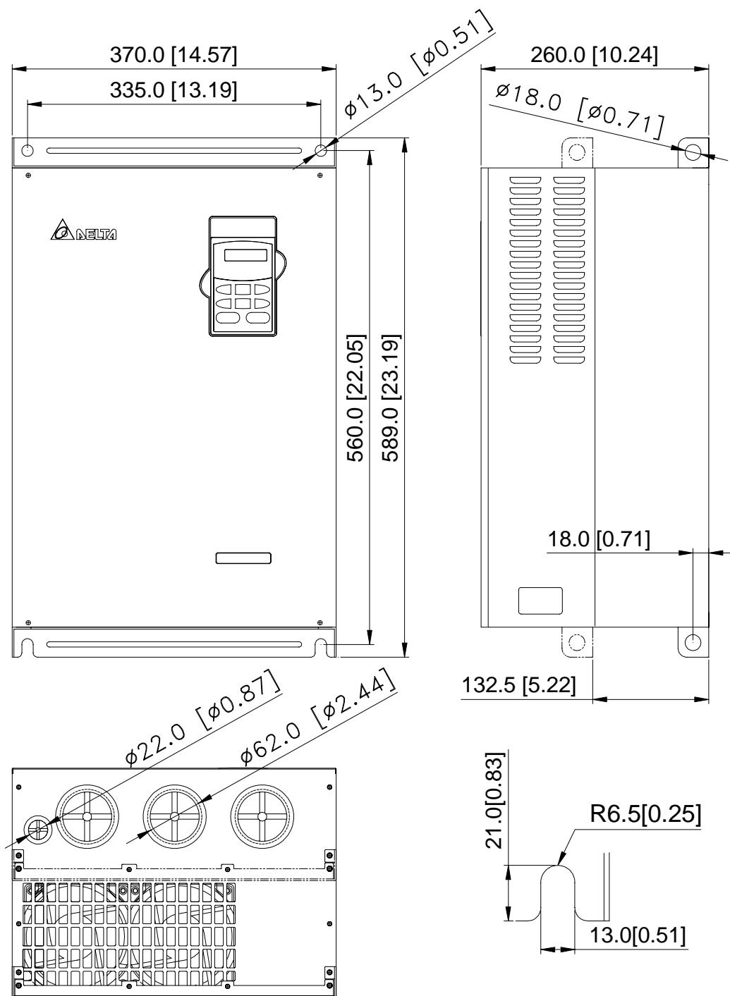
**Типоразмер Е1:** VFD300B23A, VFD370B23A, VFD550B43C/53A, VFD750B43C/53A
