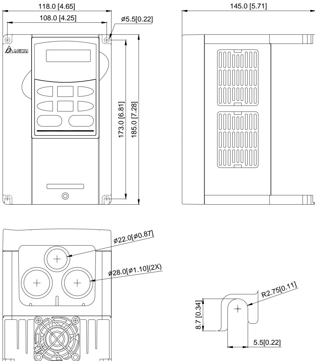
**Типоразмер В:** VFD022B21A, VFD037B23A/43A/53A
